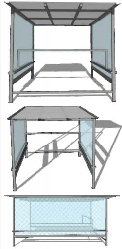
Each our structure is adapted to the weather conditions prevailing in the specific area basing on wind and snow maps.
